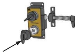
**1** Key from isolation interlock is inserted to AIE.
