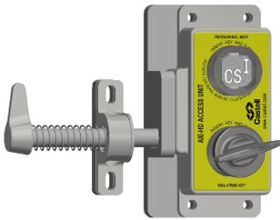
While the door is closed, the isolation key is free, the personnel key trapped in the AIE-HD, and the bolt of the AIE-HD is trapped in the mechanism.
