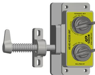
By inserting and turning the isolation key in the AIE, the personnel key can be turned and released. This traps the isolation key, which enables the release of the side bolt. The personnel key should be returned by the operator while in the hazardous area.
